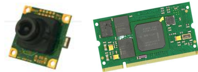
IDS-UI-1646LE-C CMOS Camera (left) Colibri PXA270 Microprocessor (right)
