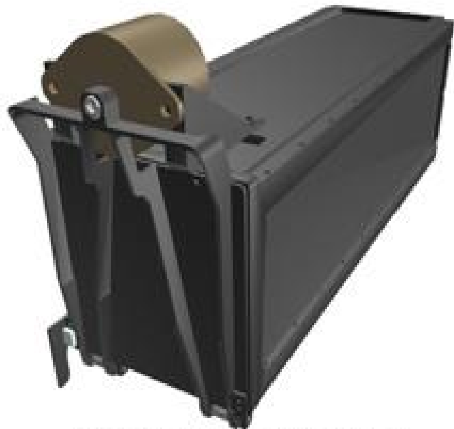
Poly Picosatellite Orbital Deployer (P-POD)
