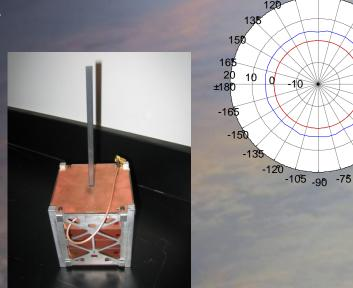
Both antennas constructed of spring steel with a Kynar cover
