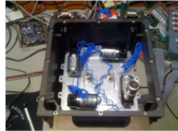
Micro Propulsion Module and P-POD test fit
