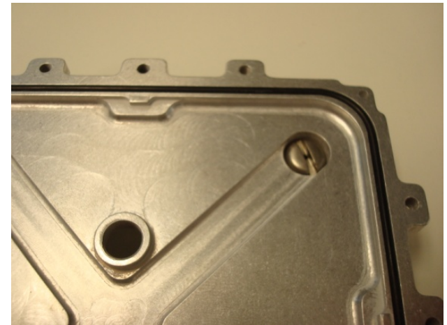
Underside of cap with stud installed
