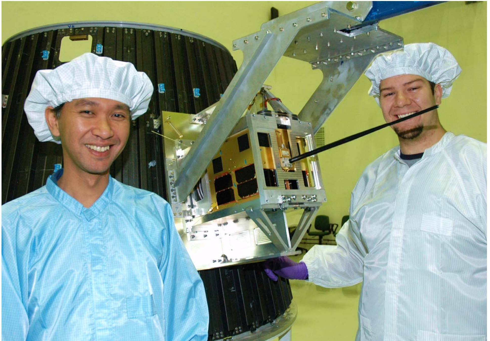
April 17: L-11 – NLS-5 is mounted on the PLA
