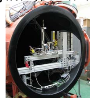
HmNT Feedsystem installed on JPL Milli-Newton Thrust Stand
