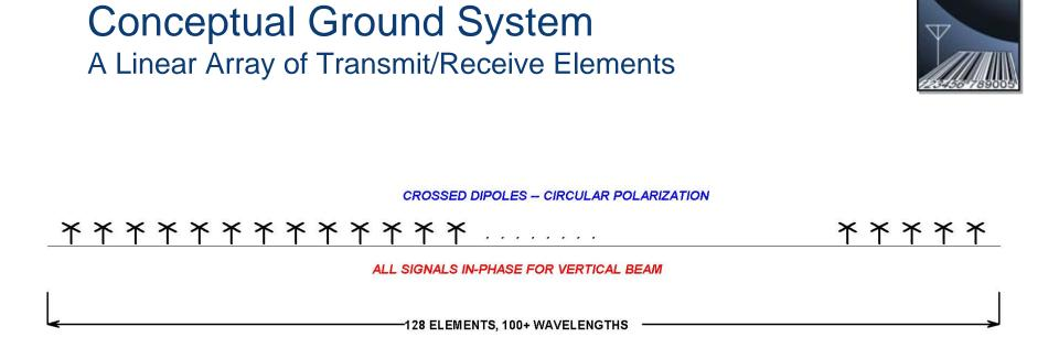
Transmit Fan Beam Array: 2 kW transmitted [16 W per element],  $0.5^{\circ} \times 120^{\circ}$  beam shape
