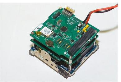
A selection of CubeSat Kitcompatible internal modules under development at Stanford's SSDL.
