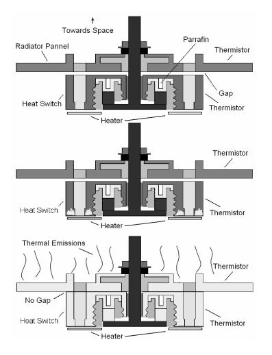
Thermal switch when open (top) and closed (bottom)
