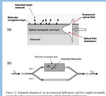
Figure 21. Schematic diagram of (a) an evanescent field sensor, and (b) a simple waveguide circuit where the sensor is incorporated into a Mach-Zehnder interferometer.
