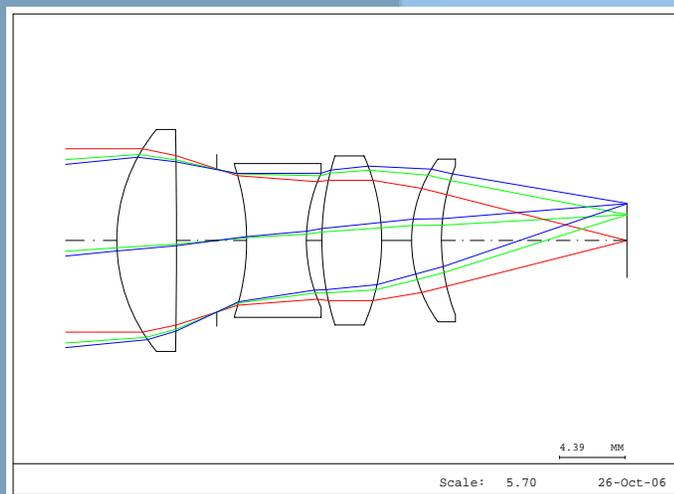
Refractive objective based in a modified Cooke Triplet
