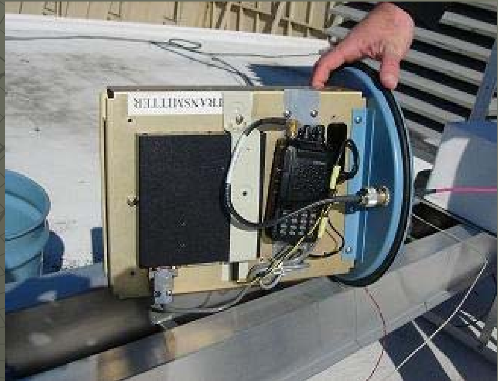
Our RF prototype on Roof
