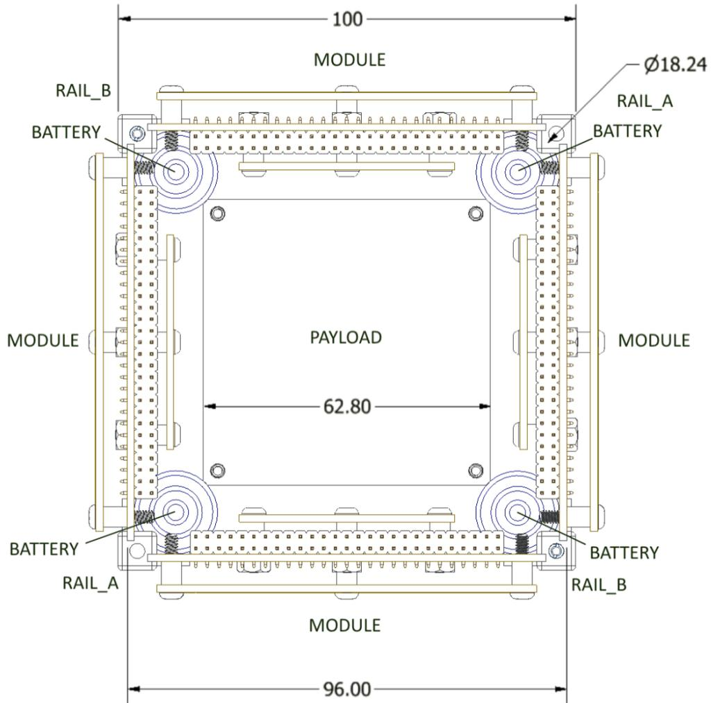
Figure 3. Diagram of the OPEN design (all units in mm).
