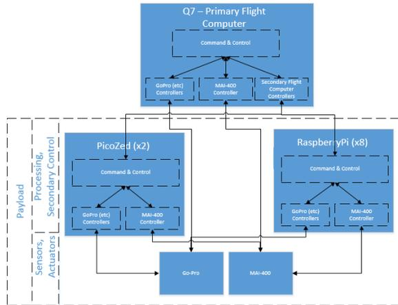
**Figure 3: ACES-RED#1 Redundant Control**
