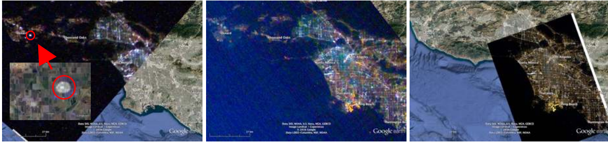
Figure 3. Two AC-5 Images of the Los Angeles region and one ISS photo overlaid on Google Earth. From Left to right: 19 Sep 2015 AC-5 NFOV Camera ~ 130m resolution GSD, 22 Aug 2016 AC-5 NFOV Camera ~ 130m resolution, 30 Nov 2010 ISS Nikon with 180mm lens ~ 20 m GSD.
