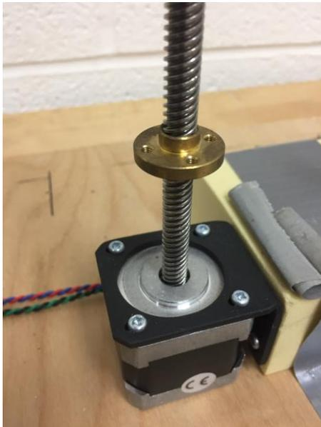
**Figure 7. Stepper Motor with Threaded Shaft and Mounting Nut**
