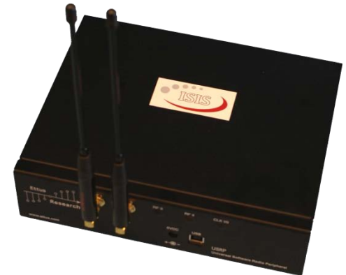
Ground station Transceiver
