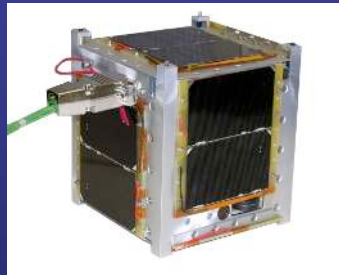
Montana Earth Orbiting Pico Explorer (MEROPE); a hand-held satellite
