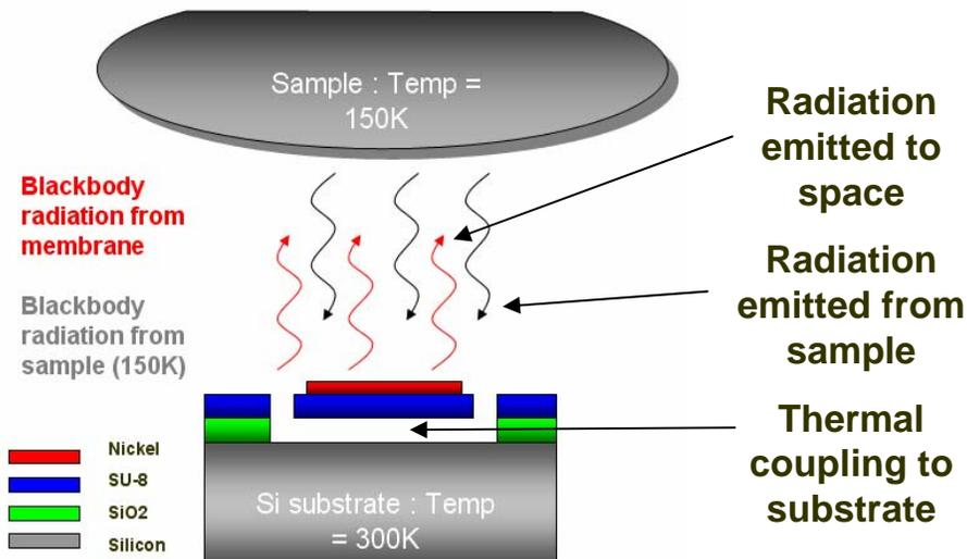
Sensitivity of 7 nV/K, but 60 nV noise floor limits resolution to 9 K
