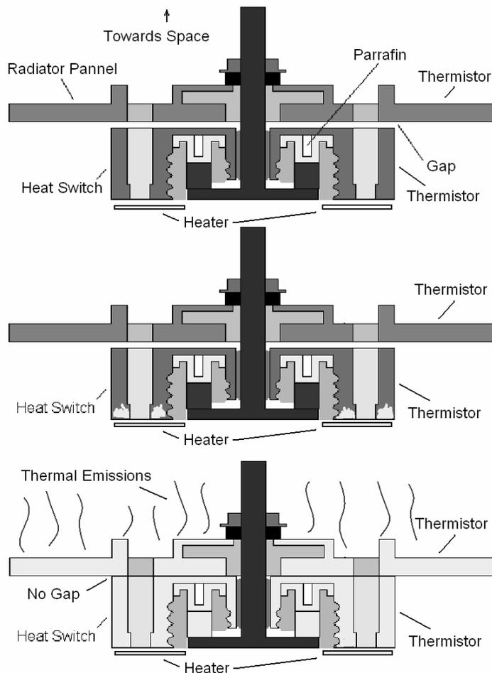
Thermal switch when open (top) and closed (bottom)
