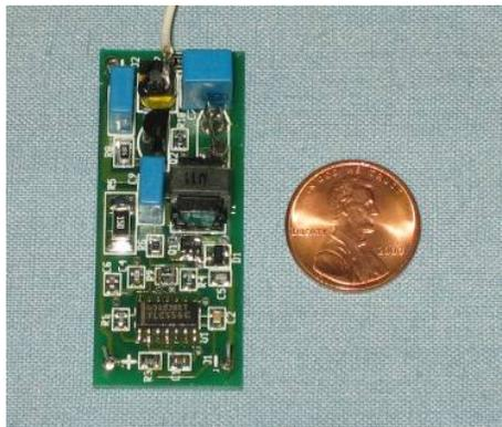
Prototype Power Processing Unit
