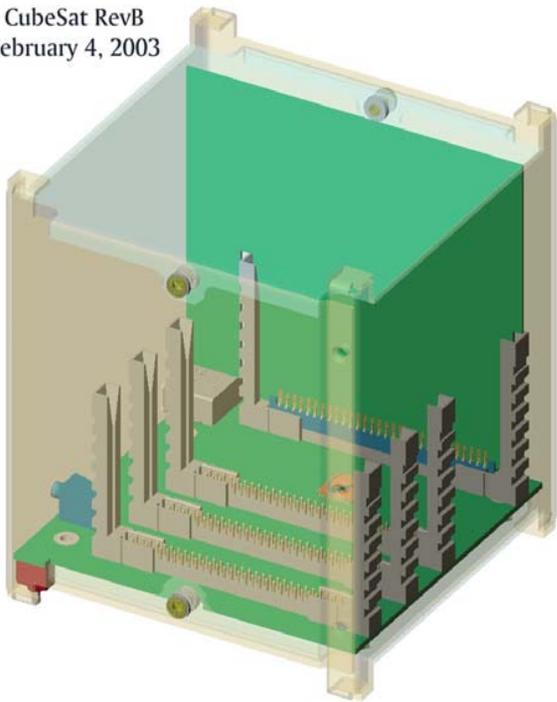
By adopting a PC/104-centric connector scheme for the CubeSat Kit, our customers are able to use components
