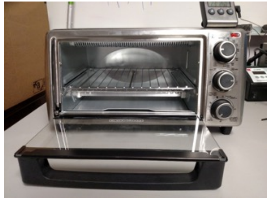
Fig. 9 High-Tech Solder Reflow Oven with added Temperature Monitor
