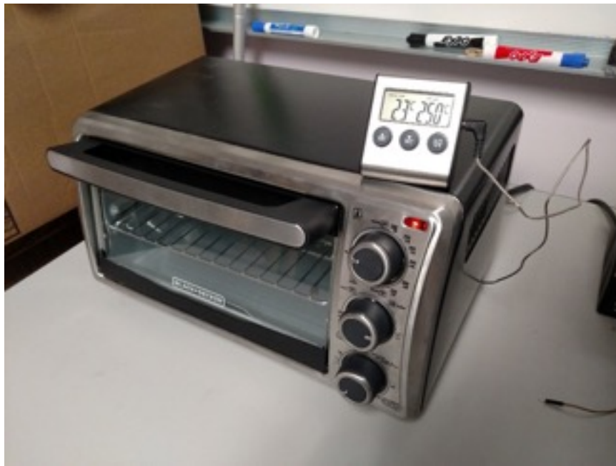
Fig. 9 High-Tech Solder Reflow Oven with added Temperature Monitor
