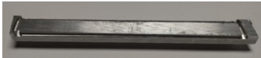
Fig. 12 Test Milling of Aluminum CubeSat Post
