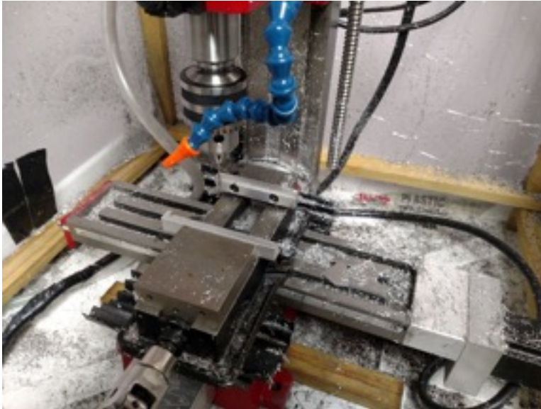
Fig. 11 Custom CNC Drill for Aluminum Frame Milling
