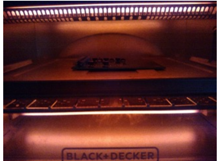
Fig. 10 PCB in the Reflow Soldering Process
