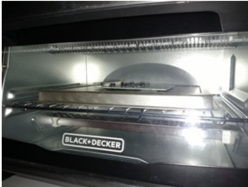
Fig. 10 PCB in the Reflow Soldering Process
