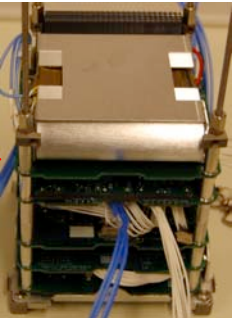
Electrical Power System + Battery Board
