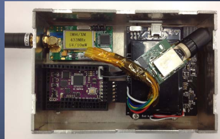
IMU / GPS Telemetry Test Unit
