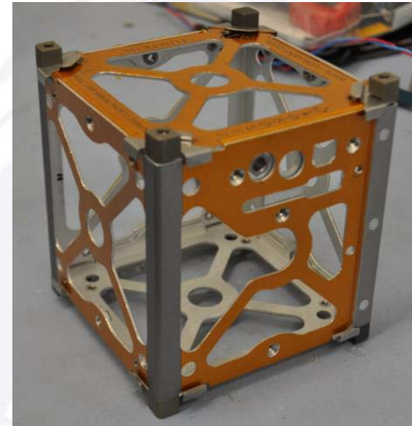
DragonSat-1 structure with Kapton tape coating on outside
