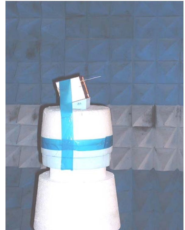
CubeSat mockup testing with whip antenna
