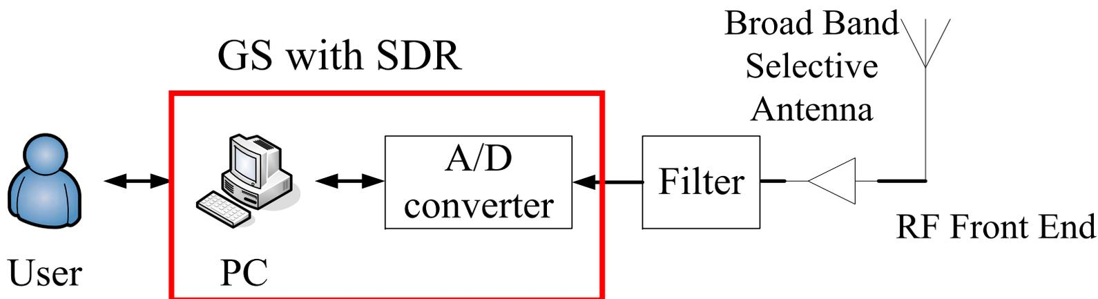
A Software Defined Radio (SDR) system is a radio communication system where components that have typically been implemented in hardware (i.e. mixers, filters, amplifiers, modulators/demodulators, detectors, etc.) are implemented using software. While the concept of SDR is not new, the rapidly evolving capabilities of digital electronics are making many processes that were once only theoretically possible practical.
