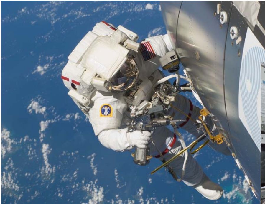
Randy Bresnik installing AIS antenna on Columbus module—Nov 2009
