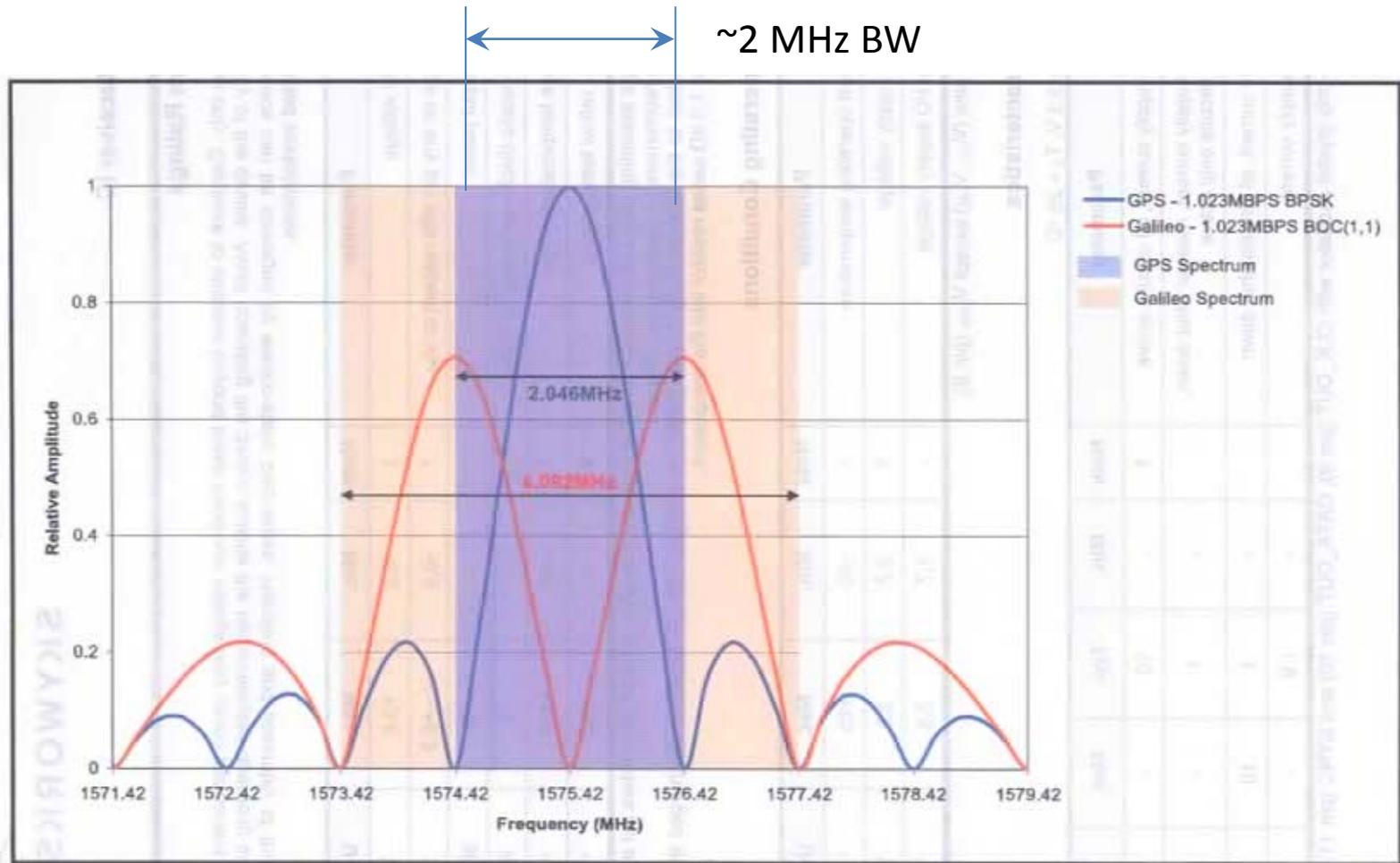
The GPS signal is a Binary Phase-Shift Keying (BPSK) modulated spread spectrum signal with a chip rate of 1.023 MSPS.
