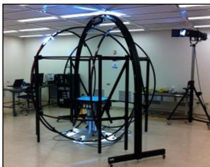
Attitude Control Test Facility ADCS testing for 1-100 kg satellites
