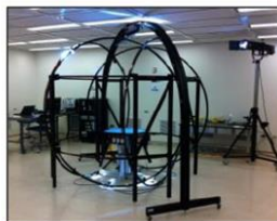
Attitude Control Test Facility ADCS testing for 1-100 kg satellites Magnetic Field, Sun, Nadir, GPS and Star tracker stimulators
