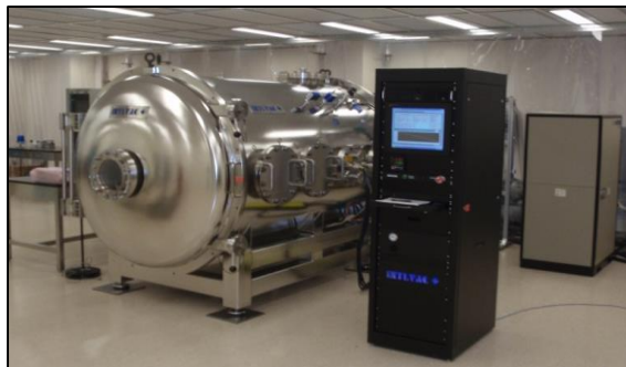
Intlvac Thermal Vacuum Chamber 1.6 m I.D. x 2.25 m long, 10^{-8} Torr
