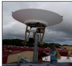
HSFL UHF/VHF/S-band ground receiving stations
