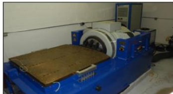
Vibration and Shock Table Tests objects 1.2 x 1.2m 5-2200 Hz to 7000 kgf; 14000 kgf shock
