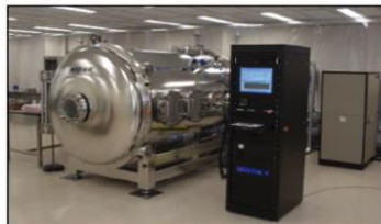
Intlvac Thermal Vacuum Chamber 1.6 m I.D. x 2.25 m long, 10^{-4} Torr
