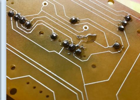
Figure D. Broken trace.
