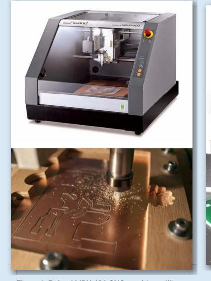
Figure 1. Roland MDX-40A CNC machine milling a PCB..
