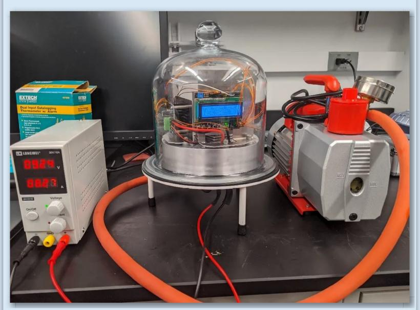
Figure 7. DIY student-safe TVAC chamber.
