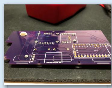
Figure F. Soldered components on purple PCB from OSH Park.
