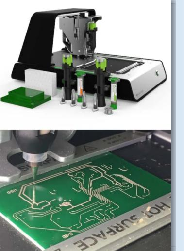
Figure 2. Voltera V-One printing conductive ink traces.
