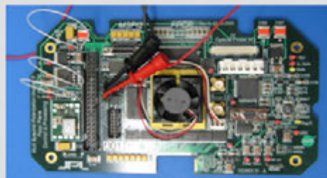
AirMSPI board with military-grade Xilinx Virtex-5 FPGA demonstrates data reduction
