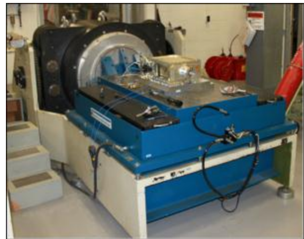
Wallops 6U Deployer during vibration test
