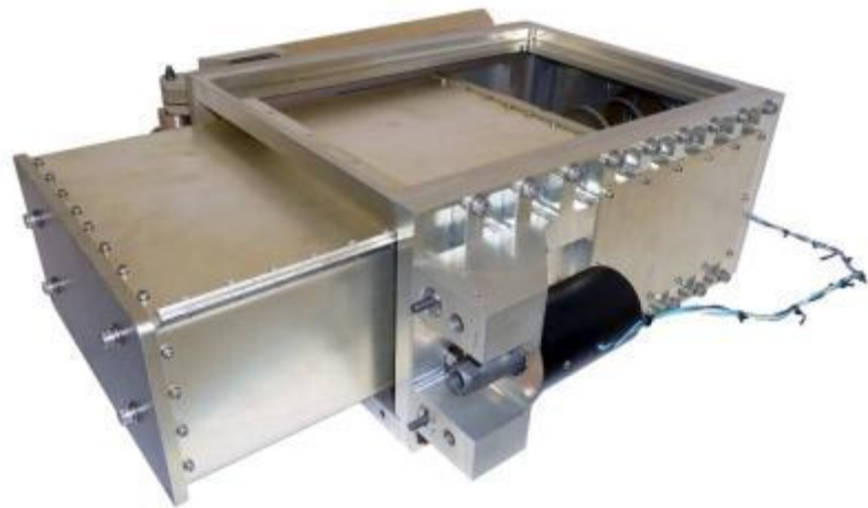
Wallops 6U Deployer with mass simulator
