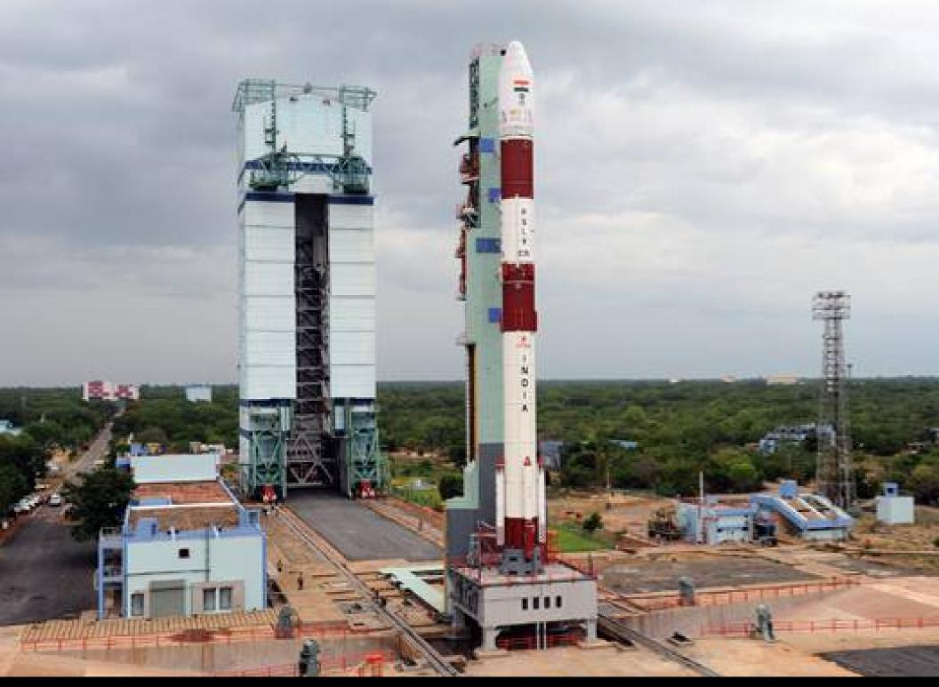
PSLV C-15 after the Mobile Service Tower (MST) has rolled back
