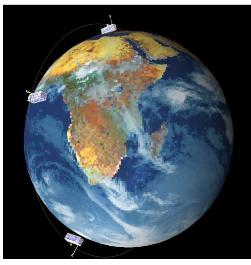
Nominal Controlled Attitude: Orbit Normal Alignment of Long Axis
