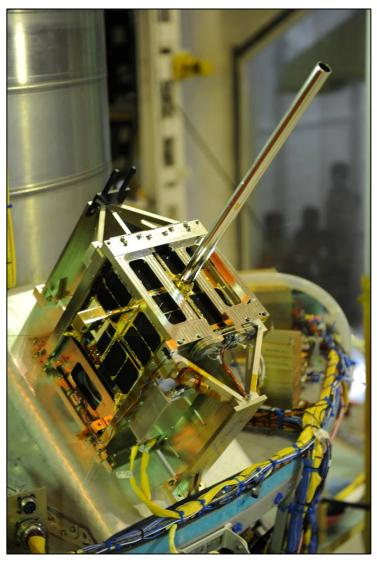
AISSat1-1 and XPOD-15G Mounted to the EB Deck
