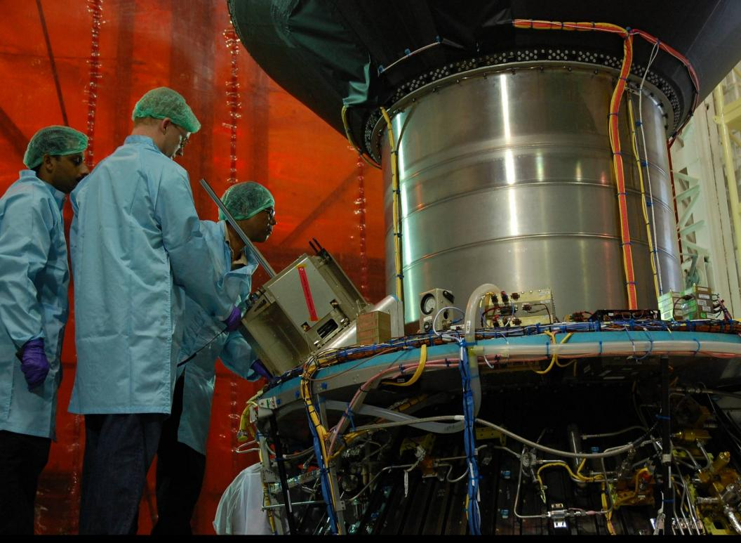
Mounting of AISSat-1 and its XPOD on the PSLV EB Deck
