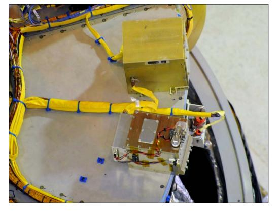
**TIsat-1 and XPOD Mounted to the EB Deck**
