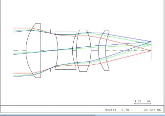
Refractive objective based in a modified Cooke Triplet
