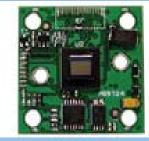
1/3" CMOS SENSOR Power consumption: < 320 mW Dimensions:28.8x28.8x5.6mm
