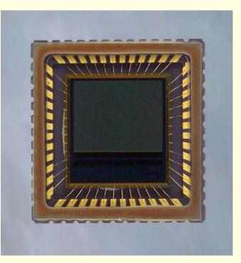
5 MP CMOS Sensor Power supply : Analog 3.3V ±5% Power Dissipation: 150mW dynamic 500µW standby
